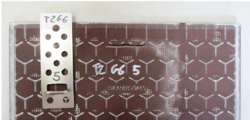
Figure 10. Hook failure mode in the G6 configuration
