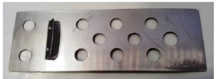
Figure 28B. 8 mm RAIFIX hook with scratches made intentionally
