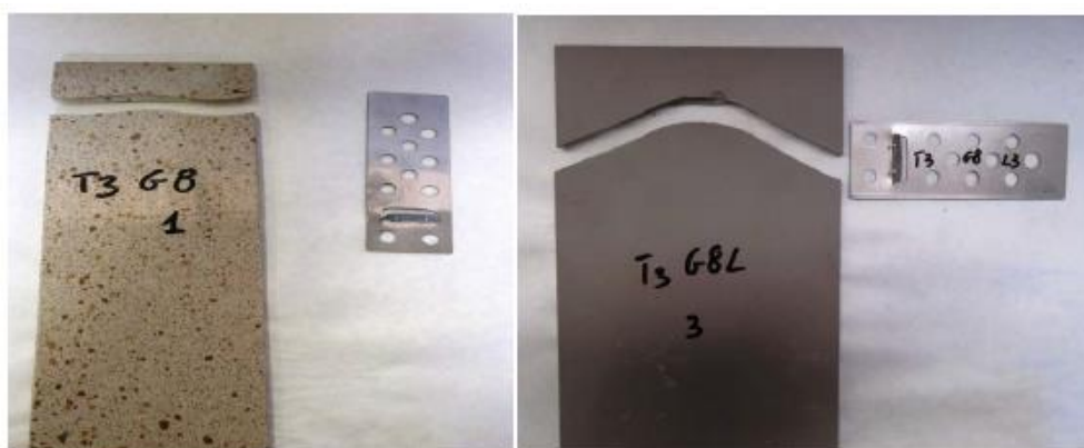
Figure 22. Failure mode in the G8 configuration
