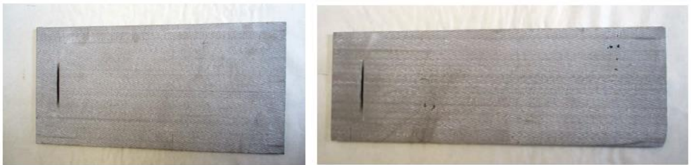
Figure 19. Example of 15 and 10 cm wide samples notched along the centre line
