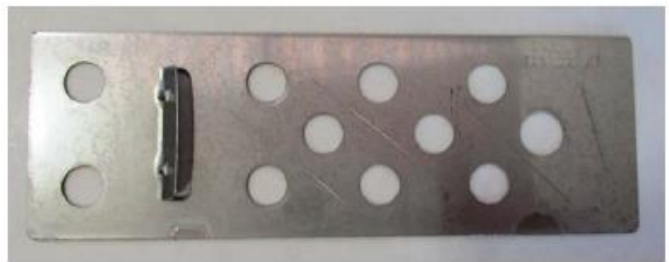
Figure 27B. 6 mm RAIFIX hook with scratches made intentionally
