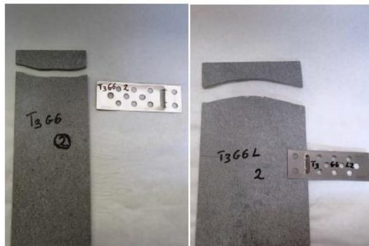
Figure 21. Failure mode in the G6 configuration
