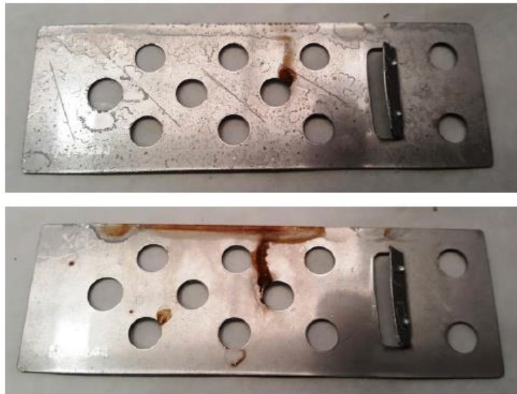
Figure 29. Samples with rust formation
