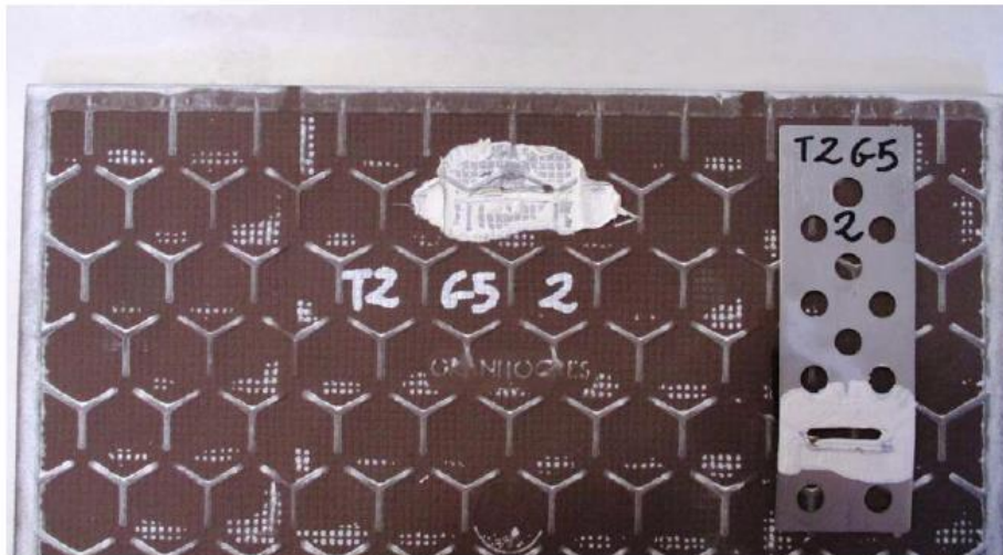
Figure 9. Hook failure mode in the G5 configuration
