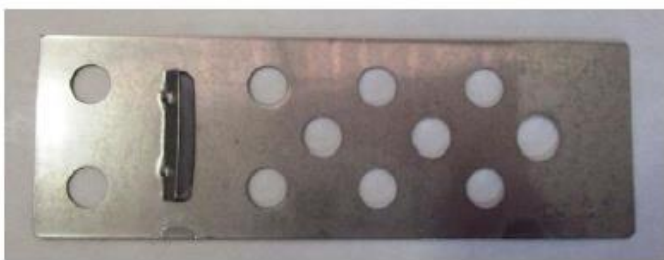
Figure 27A. RAIFIX 6 mm hook in normal (intact) condition
