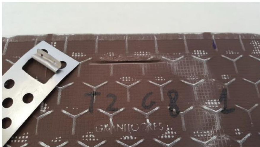
Figure 11. Hook failure mode in the G8 configuration
