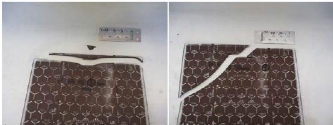
Figure 18. Hook failure mode in the G8 configuration (left: 15 mm; right: 30 mm)
