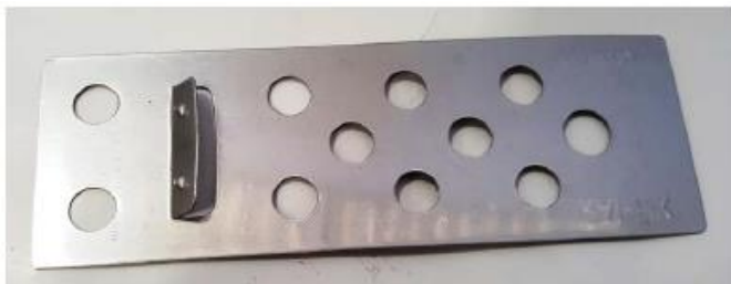
Figure 28A. RAIFIX 8 mm hook in normal (intact) condition
