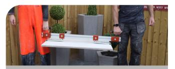
Slab lifters help move flags around safely. Iwo-man slab lifters are ideal for those heavier flags. The two man slab lifters can be used in pairs for even safer lifting of large slabs.
